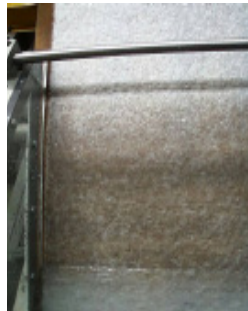
T-153 shortcut fibers in a wetlaid web formation process.
