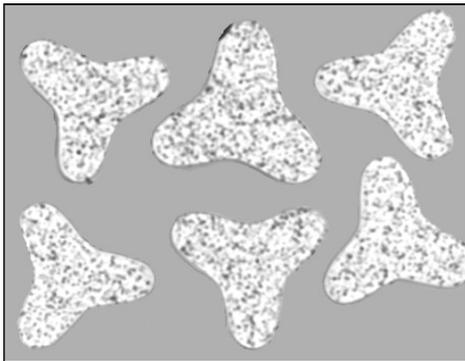
FiberVisions trilobal staple fibers allow customers to make nonwoven fabrics with dramatically improved coverage and uniformity while maintaining equivalent fabric strength and softness. Additionally, these fibers can be supplied in both a standard and a high opacity version. Furthermore, these trilobal fibers are optimized for dry laid nonwoven formation systems and are specifically designed to be converted into carded thermal bonded (CTB) fabrics.
