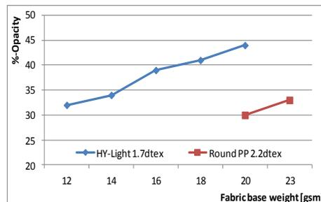
The increased surface area of the fibers results in higher light scattering and therefore, higher opacity.
