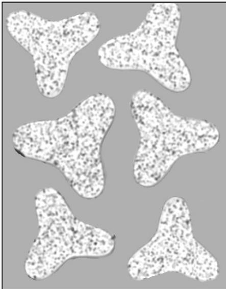
FiberVisions trilobal PP staple fibers allow customers to make nonwoven fabrics with dramatically improved coverage and uniformity. Additionally, these trilobal fibers have been produced at finer titers to improve nonwoven softness and strength and further improve coverage and uniformity versus round staple fibers.
