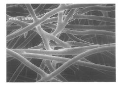
Optimum fiber properties are achieved by combining the physical properties of the fiber with our advanced finish technology. This gives outstanding liquid acquisition performance in the nonwoven.
